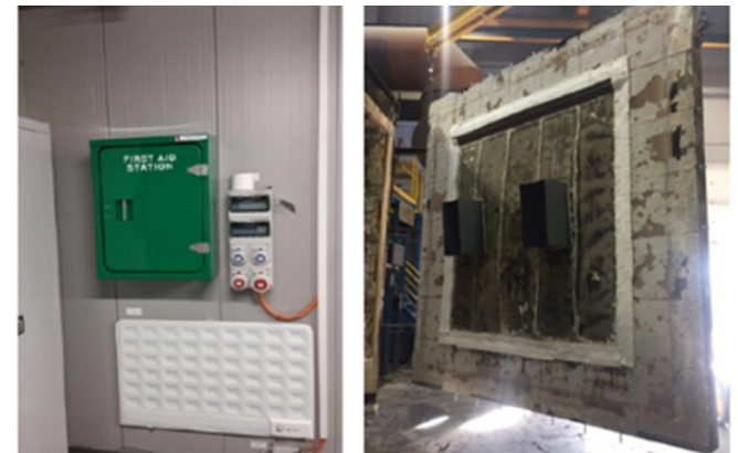
Figure 15 Left, equipment installed on Generation IV internal sandwich wall panels, within limits of A60 certification. Right, 5x66 pounds (30kg) equipment mounted on sandwich panels during fire test, 3 on cold side and 2 on hot side.
