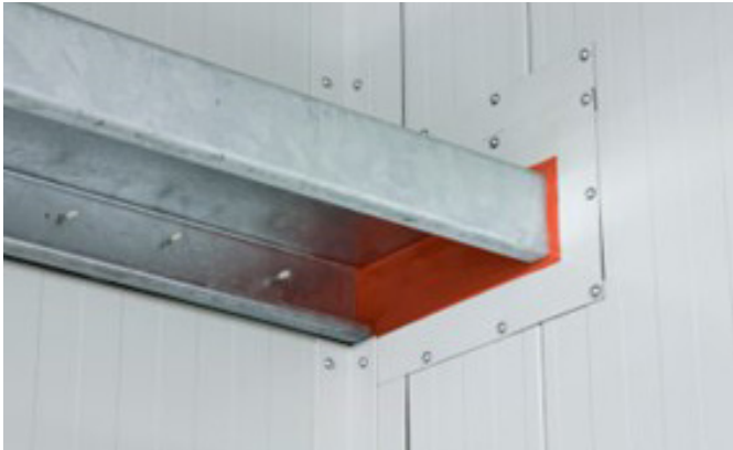
Figure 10 C profile for mid span support of large (over 20 ft long) Generation IV A60 external sandwich panel wall. The C profile penetrates an A60 internal Generation IV sandwich wall and is A60 certified closed with Nofirno.
