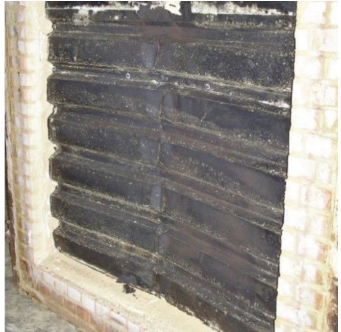
Figure 25: Type III wall exposed side after 1.0 bar blast and prior to H120 fire H180 fire
