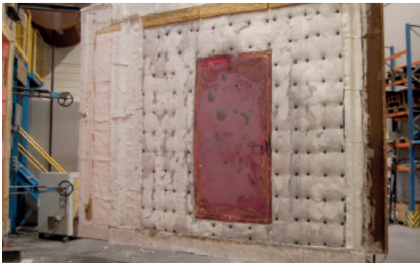
Figure 27 Test specimen following the test, seen from the exposed side.
