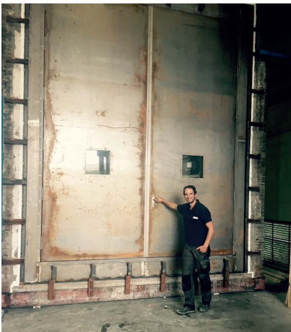
Figure 3 Double hinged XL door 4200 x 3250 mm (HCO x WCO) A60 certified.
