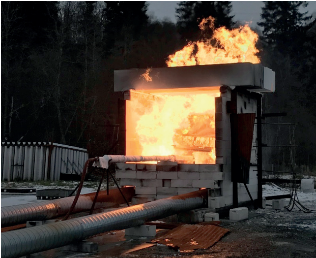
Figure 2 J15 HHF test on NORSOK approved sliding door.
