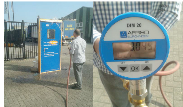
Figure 6 Weather-tightness test of hinged door according to Norsok C-002 [4].
