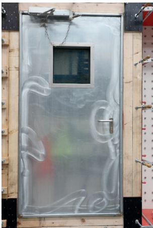
Figure 4 Gas tightness test.
