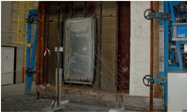
Figure 26 Test specimen 240 min into the fire test.
