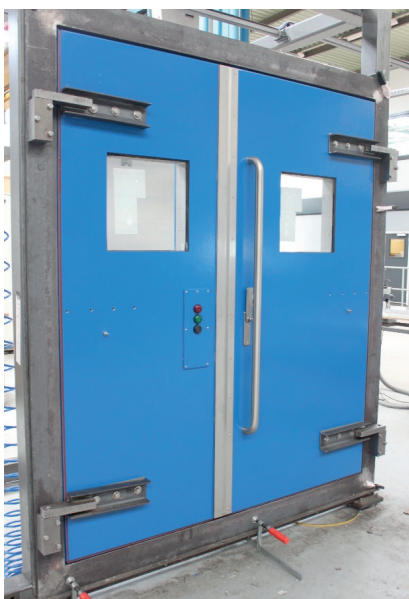
Figure 12 H120 1.6 bar blast door, blast, fire and usage category I for main entrance of control room, including hydraulic door closer and access control.
