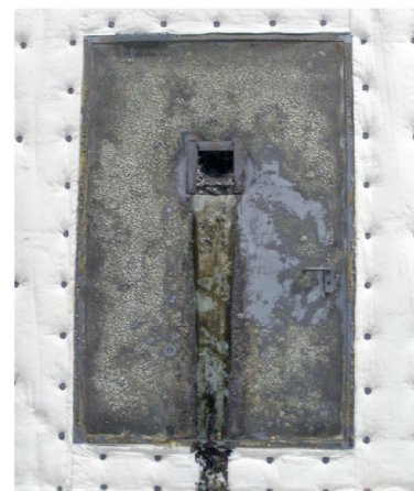
Figure 29 H120 fire door test including a 200 mm x 200 mm vision panel, seen from the exposed side (several glass layers melted during the test).
