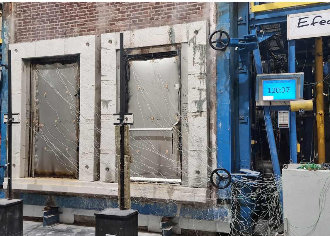
Figure 6: InterDam Hinged doors tested at Effects on fire resistance from both sides at same time.
